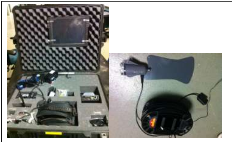
Figure 4. Underwater video camera manufactured by SeaViewer and used in Florida surveys. Equipment in the left pane is self-contained data acquisition equipment with integrated screen, GPS (for overlay on the video, and Bluetooth glasses to visualize the video while traversing the bottom. Pane on the right is the camera and cable. Data is saved to an SD card which is read using standard video editing software.
