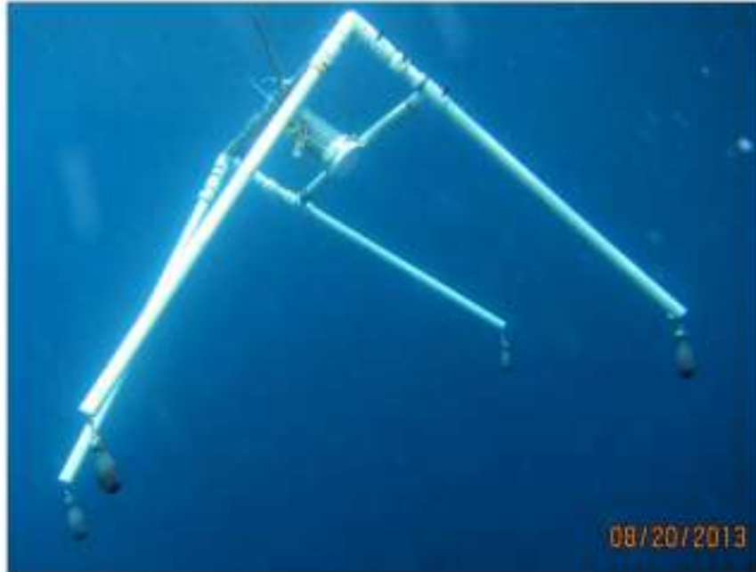
Figure 5. Photograph of deep water survey showing set up of submersible live-action SeaViewer underwater video camera rigged with weighted PVC cradle
